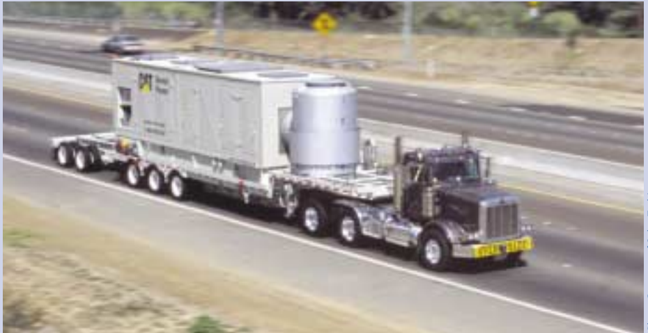
The Taurus™ 60 Mobile Power Unit (5.5 MW) from Solar Turbines features a modular design with plug-in connections for rapid set up. It is easily transported over land as shown above.
